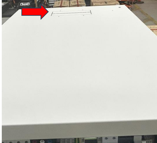
Figure 7 – Top Cable Entry Details
