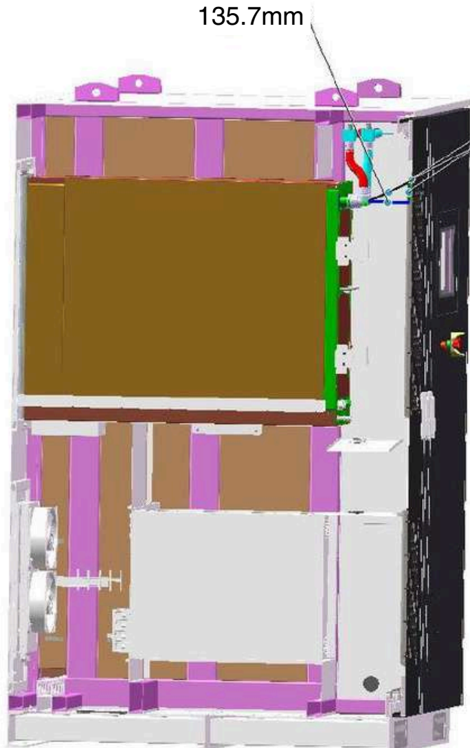
Distance between liquid cooling pipeline and front door: 135.7mm
