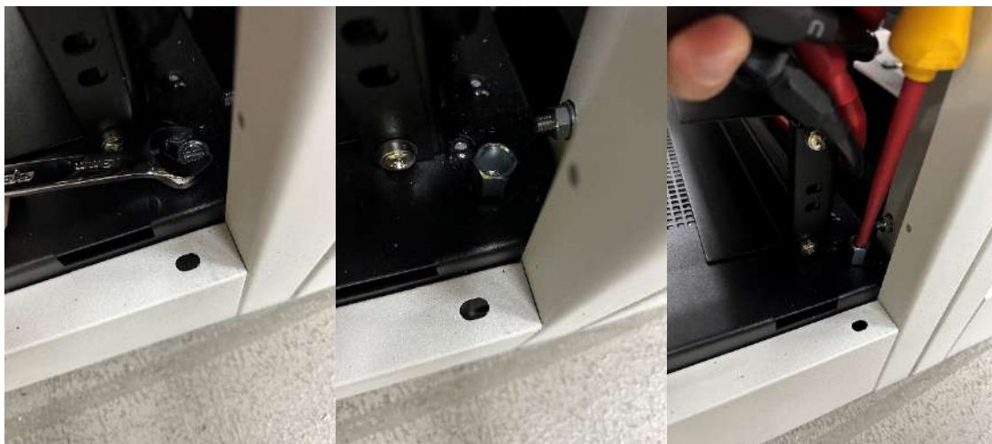
Figure 6 – ESCA2028-1XX Cabinet Adjustable Legs and Castor Wheels
