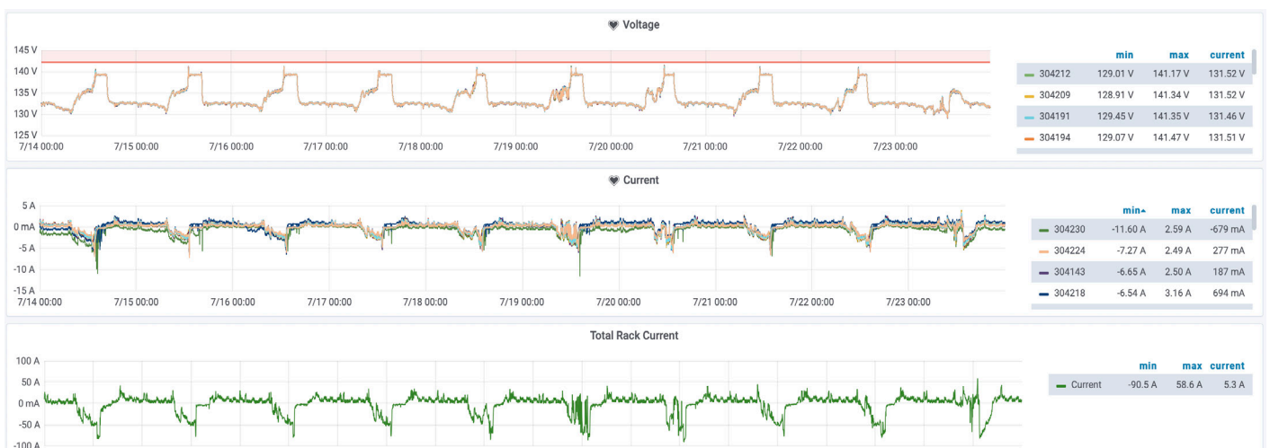
Screenshot displaying types of information accessible through the Powerlink from LiFe12033P.
